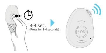
When you need help, press the SOS button for 3-4 seconds till you hear a voice prompt of activating an SOS alarm. Your device will also vibrate at this time.
